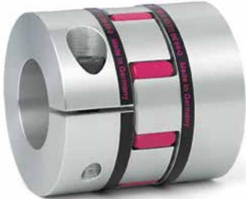
This elastomer insert transmits torques ranging from 0.5 to 25,000 Nm at zero backlash and compensates for axial, lateral and angular shaft misalignments. It enhances the entire drive train and delivers damping capability, torsional rigidity and thermal stability. This damping capability is particularly important in systems and equipment subject to frequent impact, reversing, or vibratory loads.
