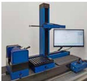
Contourgraph testing is an integral part of the quality assurance process for components featuring complex, yet essential-to-functionality geometries. That is why safety coupling components in particular undergo this process.
